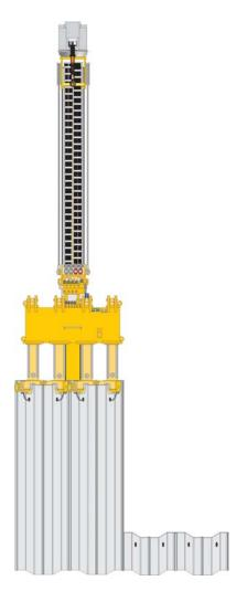
All piles pressed individually to the same level. The stroke on each pressing unit is 450 mm.
